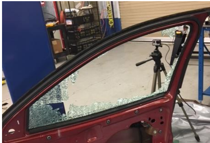
Figure 16: Results of tool no. 4 test on tempered glass. Image Source: AAA
